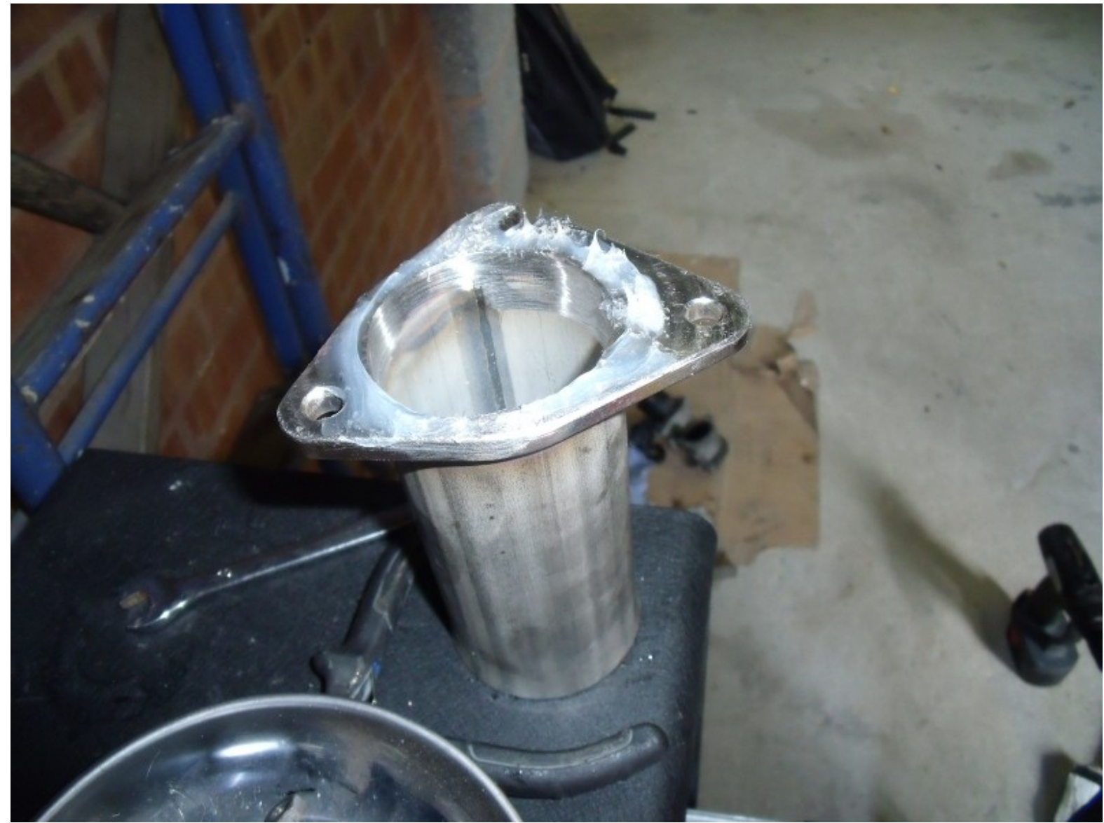
Fit using stainless M6 x 16mm panhead bolts and washers for a neat look...
